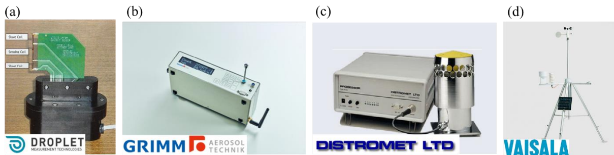
Figure 3.2 The pictures of the instruments, (a) LWC-300, (b) Aerosol Spectrometer (MODEL 11-D), (c) JWD, and (d) Automatic weather station.
